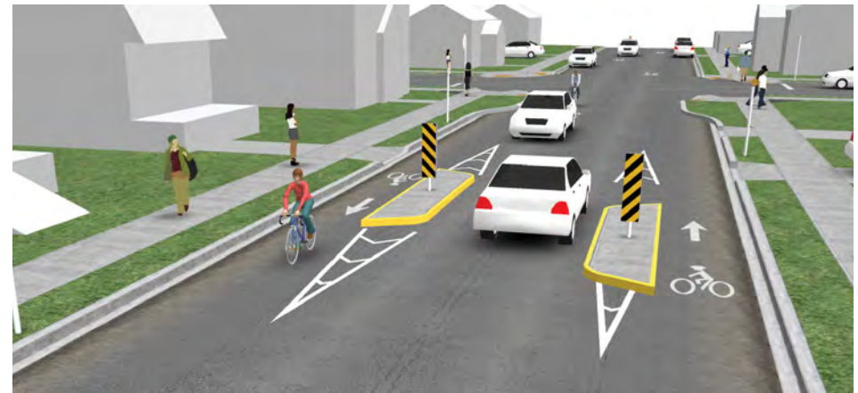
Top Image: Chicanes are used to slow speeds near a park (Boise, ID); Middle Image: Choker or pinchpoint graphic by NACTO;
