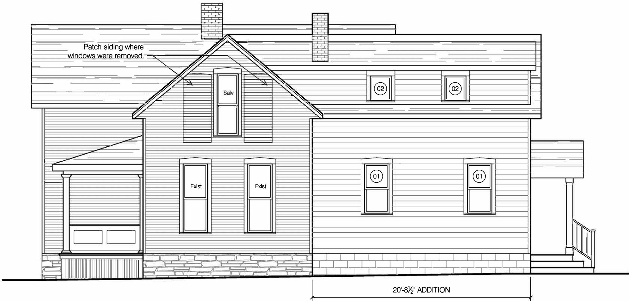
A5 NORTH ELEVATION - NEW WORK SCALE: 3/16" = 1'-0"
