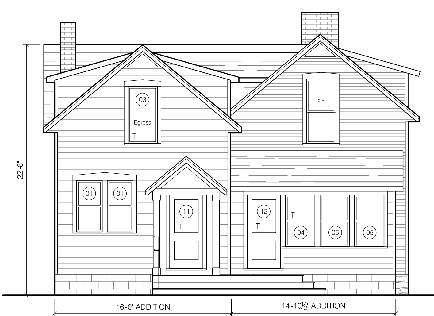
A8 WEST ELEVATION - NEW WORK SCALE: 3/16" = 1'-0"
