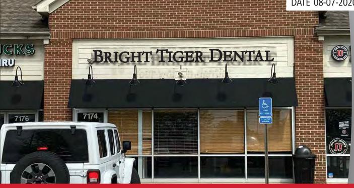
14 3/16" Internally illuminated (with white LEDS) face-lit channel letters mounted flush to fascia
